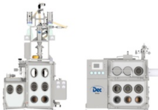
Dec PTSbased high containment handling system showing filter dryer discharge isolator (left) and pack-off and milling chamber (right)
