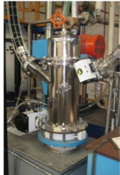
Fully sealed PTS connection to reactor
