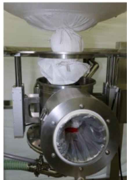
Dec SafeDock: power-free safe docking of big bags under full containment
